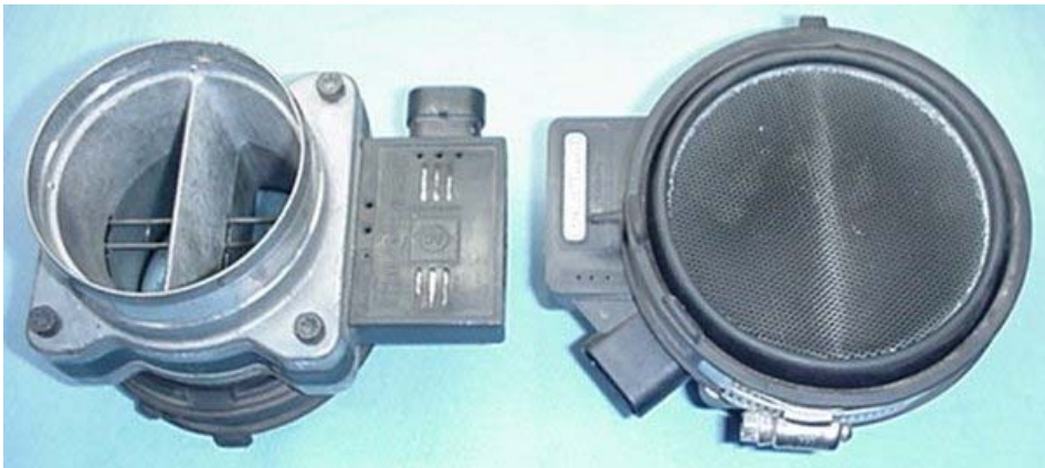
The MAF on the left (75mm) 3 pin connector, the MAF on the right (85mm- 5pin) used on later LS1, Ls6 and Vortec V8 engines.
