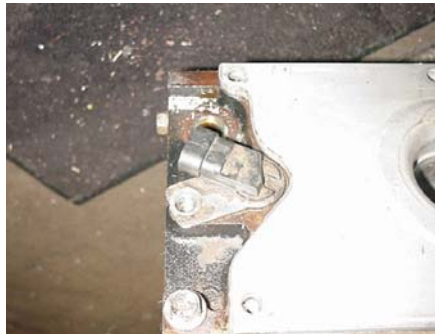
The location of the CMP is on the top rear center of block
