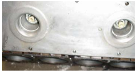
Location for the sensors is on the top of the block under the intake
