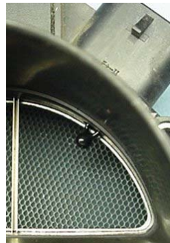
IAT sensors used in the air duct (LS1) The Vortec V8 and LS6 has the IAT integral with the MAF sensor.
