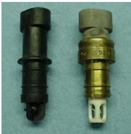
IAT sensors used in the air duct (LS1) The Vortec V8 and LS6 has the IAT integral with the MAF sensor.
