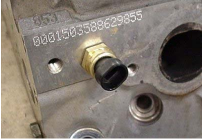
ECT location in the front of driver's side cylinder head.
