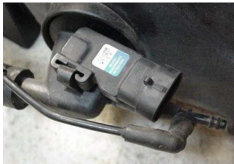
Typical MAP sensor used on many post' 96 GM cars. Location of the LS1/LS6 MAP sensor, Vortec V8's located on top of intake.
