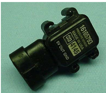
Typical MAP sensor used on many post' 96 GM cars. Location of the LS1/LS6 MAP sensor, Vortec V8's located on top of intake.
